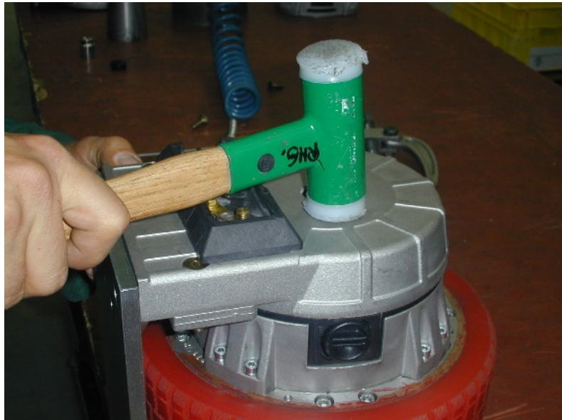
13. Put on brush flange straight to the drive motor shaft
